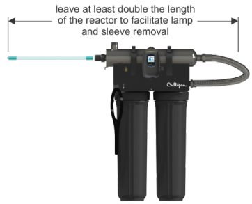
Figure 3. Lamp Removal Spacing
